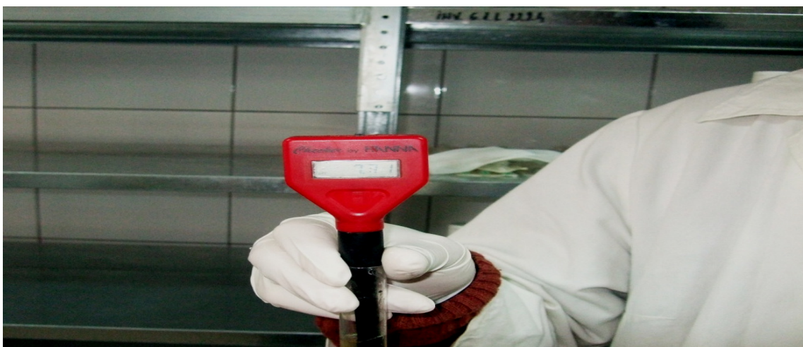
Photo 2. Determination of pH in liquid solutions - elaboration of working methodology on the use of Hanna pH meter with electronic display
